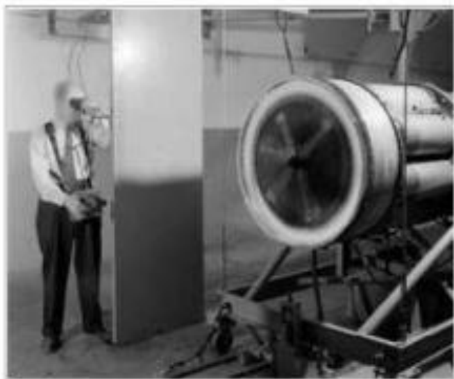
Photo: Left: A NASA scientist uses an optical pyrometer to measure the temperature of a rocket cone in a 1956 experiment. Photo by courtesy of NASA Glenn Research Center (NASA-GRC) . Right: How it works.
