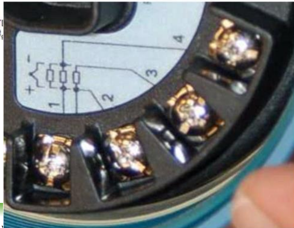
Fig.3. Two wires RTD Bridge
