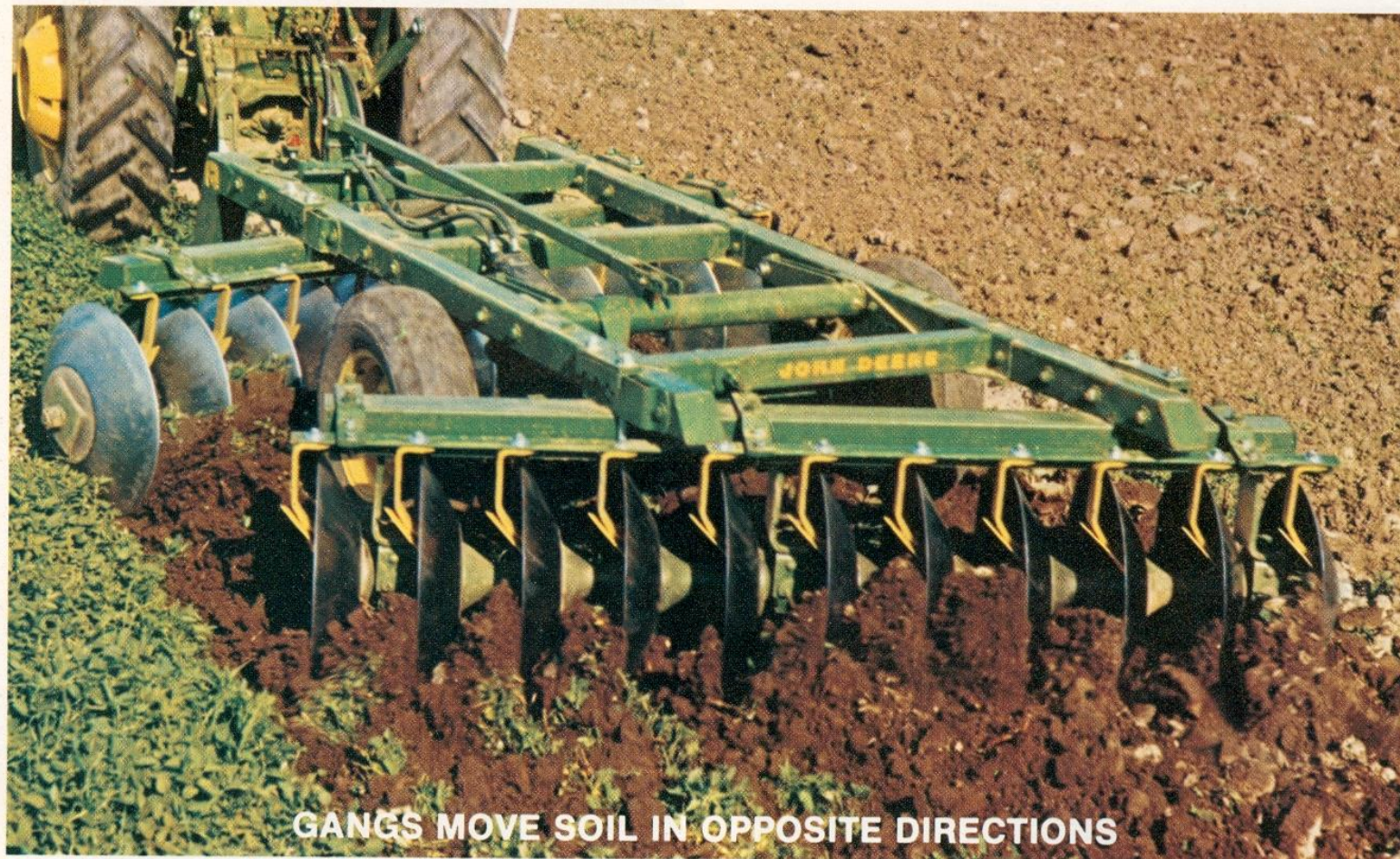
Fig. 20—Front and Rear Gangs on Offset Disk move Soil Opposite Directions
